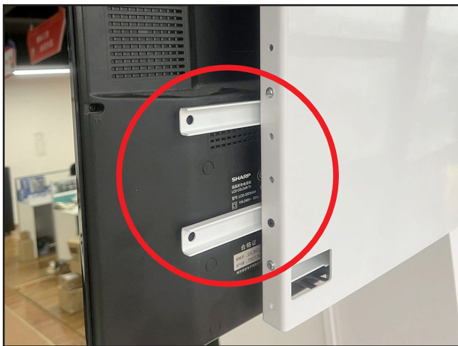
7 Slide the short VESA strips or the lift extension plate to the groove of the machine plate.
