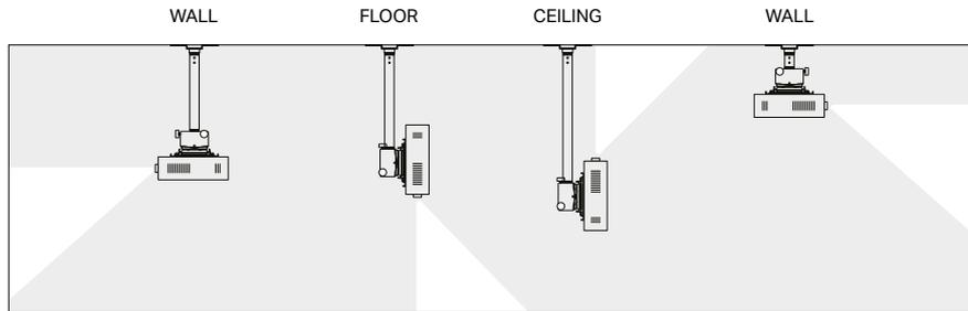
*This projector mount can be positioned to project on different surfaces such as the floor, the walls or ceiling.*
