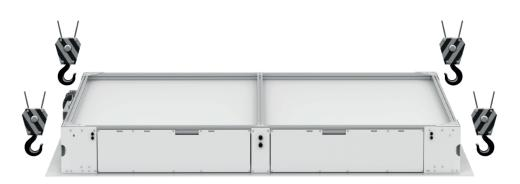
**2.** Attach the ceiling mount onto the mounting frame and lock it with four (4) screws to prevent it from slipping.
