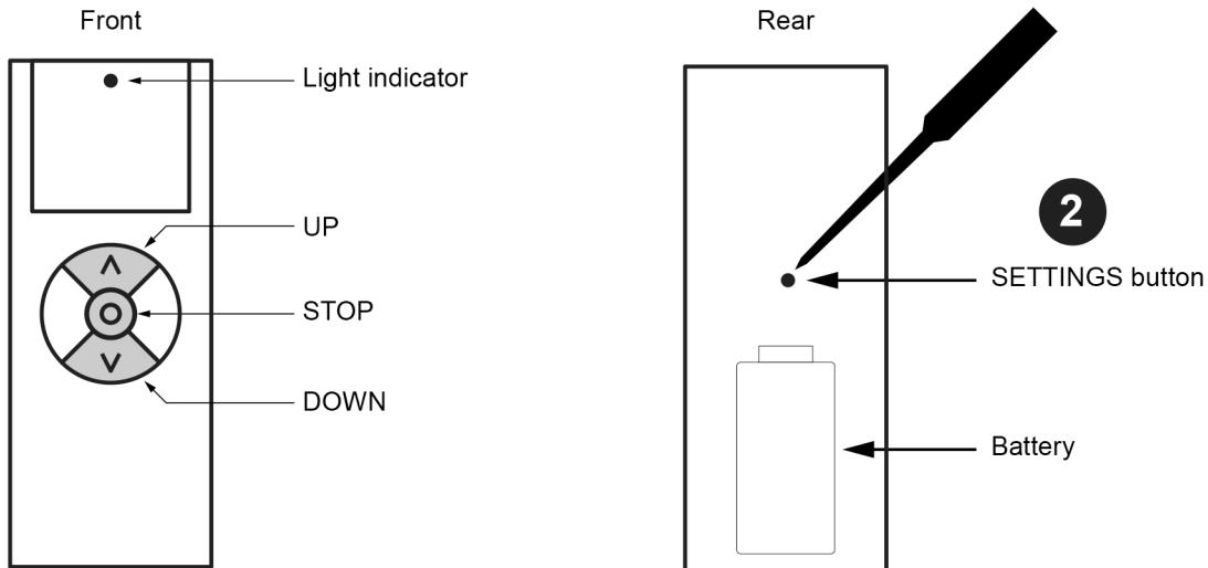
1. Press the up, stop, and down buttons of the remote control, and the TV Flip will perform the up, stop, and down actions respectively.
