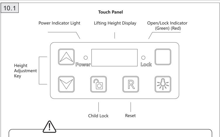
Please initialize the product under no-load condition before hanging the TV set, after powering on 100-240 V, long press the  $\mathbb{R}$  key on the touch panel to initialize the settings (see below), when the number on the touch panel reads "1750", the product can be used normally.
